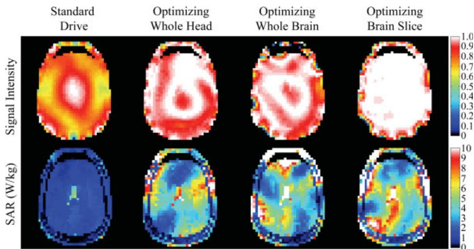
**Figure 3** Signal intensity distribution and SAR levels (in each 5-mm-cubed voxel) on an axial plane through the center of the brain for four different field distributions of interest.
