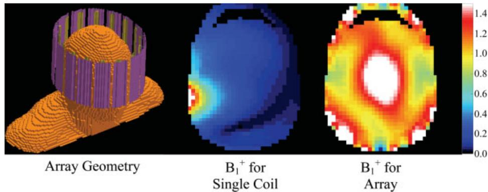
**Figure 1** The geometry of the array modeled (left) and the magnitude of the circularly polarized component of the  $B_1$  field pertinent to excitation ( $B_1^+$ ) field when driving a single coil alone (center) and when driving all coils simultaneously (right). Linear color scale is from 0 to 1.5  $\mu\text{T}$ .
