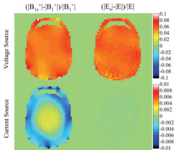
**Figure 2** Relative difference between superimposed magnetic fields ( $B_{1s}^+$ ) and superimposed electric fields ( $E_s$ ) from 16 separate field calculations (with only one coil driven in each) and their counterparts ( $B_1^+$  and  $E$ ) from a single calculation when all 16 coils are driven simultaneously. When current sources are used (bottom), the error in using superposition is seen to be much lower than when voltage sources are used (top).
