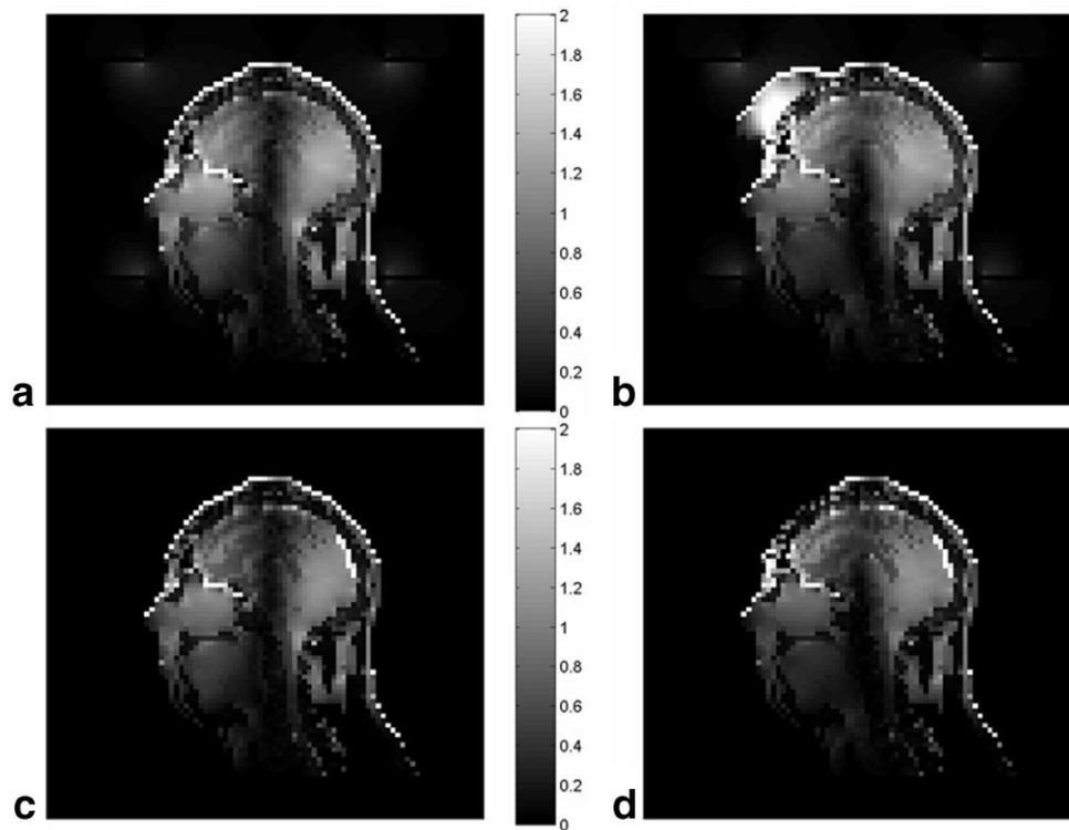
**Figure 3.** The z-component of displacement current density (**a** and **b**) and conductive current density (**c** and **d**) ( $\text{A}/\text{m}^2$ ) without (left column) and with (right column) the dielectric pad.
