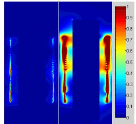
Figure 3: E field magnitude (V/m) for coils driven with (left) multiple current sources distributed throughout each coil and (right) a single voltage source placed toward the superior end (toward top of page) of each coil. Voltage source placement corresponds with location of high electrical fields in this second case.
