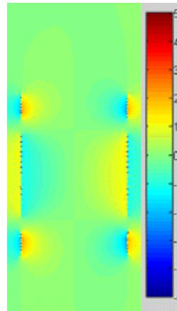
Figure 2:  $H_z$  (A/m) distribution – very similar for both driving configurations.
