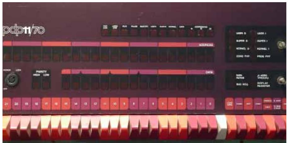
Fig 2. Front panel from a PDP 11/70 with toggle switches to allow one to enter the 'bootstrap' code to allow the machine to boot.
