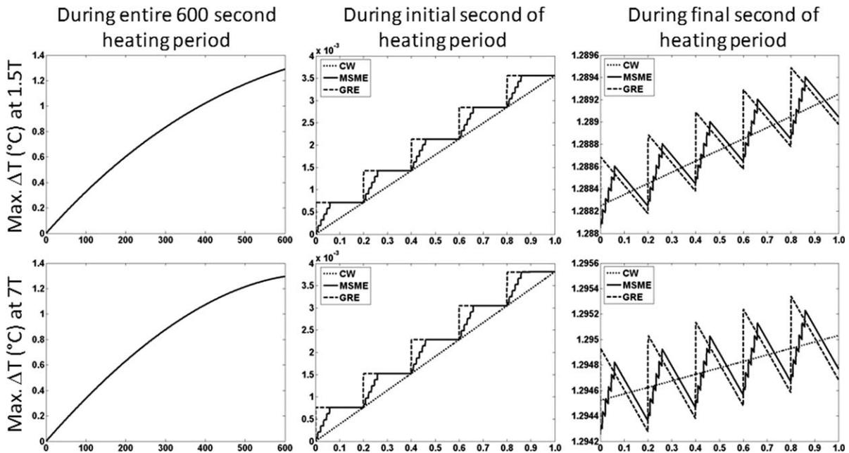
**Figure 3** The temperature rise above baseline at the location of maximum temperature change during the entire time course (left), during the first 1 s (center), and during the last 1 s (right) of a 10-min exposure to 3.0 W/kg head-average SAR at 64 (top) and 300 MHz (bottom).
