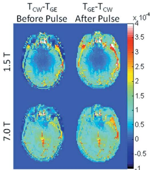
**Figure 4** Temperature difference between CW and ME sequences on an axial plane passing through the eyes immediately before (left) and immediately after (right) a single RF pulse of the GE sequence applied near the end of the 10-min period of heating at both 64 (top) and 300 MHz (bottom). [Color figure can be viewed in the online issue, which is available at [wileyonlinelibrary.com](http://wileyonlinelibrary.com).]
