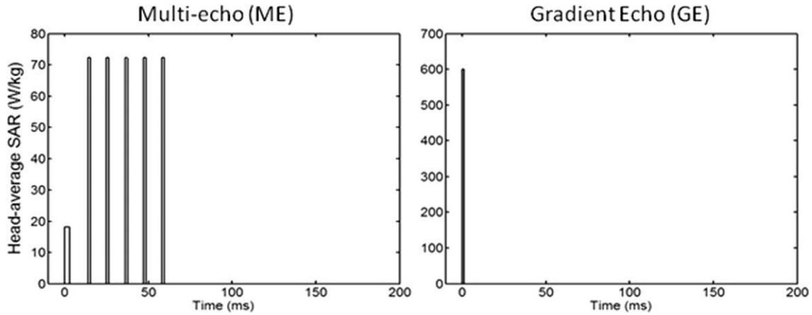
**Figure 2** Head-average SAR for different sequences simulated. Left: Multiple spin echo (ME) with TR = 200 ms and TE = 11 ms; the duration of 90° and 180° pulse is 3 and 1.5 ms, respectively. Right: Gradient echo (GE) at TR = 200 ms and pulse duration of 1 ms. Also simulated (but not shown in this figure) was a continuous-wave (CW) excitation. For all sequences, the time-average SAR over the head is 3 W/kg.
