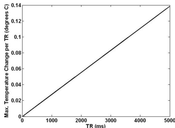
**Figure 5** Maximum change in temperature during any single repetition for a 2-h long gradient-echo sequence with a pulse duration of 1 ms and a value of TR varying from 1 (CW) to 5,000 ms in muscle tissue with time-average SAR of 10 W/kg as calculated with conservative semianalytical methods allowing for no thermal conduction.
