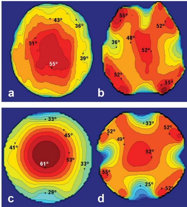
**Figure 4.** Top:  $B_1^+$  maps obtained on a human head using (a) TEM volume coil alone and (b) during the TEM/CRC array simultaneous transmission. Bottom:  $B_1^+$  maps obtained on a 3.0 L spherical phantom using (c) TEM volume coil alone and (d) during the TEM/CRC array simultaneous transmission.
