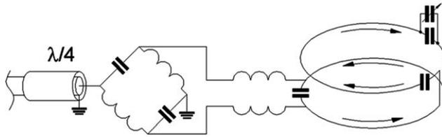
**Figure 2.** Schematic of the individual CRC coil including matching network. CRC coil is shown schematically as two circular loops (see text for details of the CRC coil geometry).
