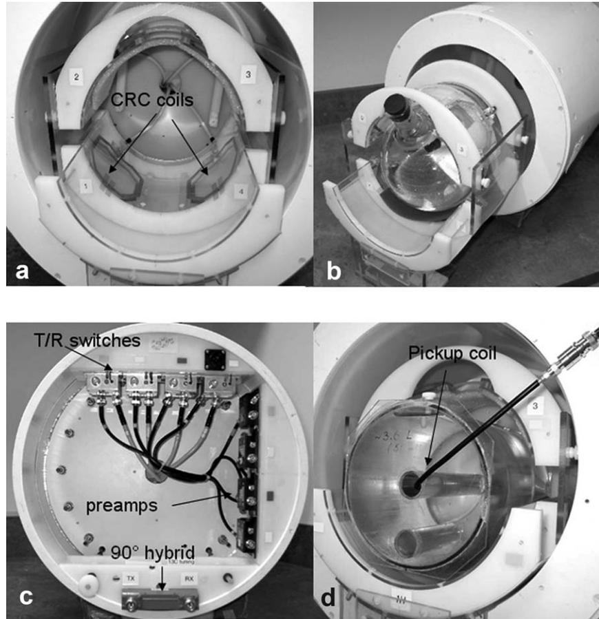
**Figure 1.** Photographs of the front side of the TEM volume coil (**a**) with the CRC phased array placed inside of the TEM and (**b**) with the array moved out of the volume coil. **c:** Back view of the TEM/CRC phased array assembly with all the T/R switches and preamplifier mounted on the volume coil's shell. **d:** TEM/CRC array assembly with the cylindrical phantom placed inside of the array. A 1-cm pickup coil was used for phase adjustment as described in the text.
