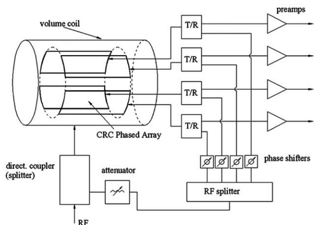
**Figure 3.** Schematic of the experimental setup for simultaneous transmission and reception with the CRC phased array and the volume coil.
