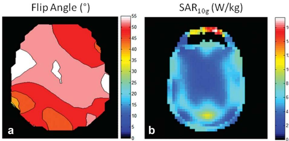
**Figure 6.** Optimum achievable  $B_1^+$  (flip angle) map on an axial slice through the center of the brain (a) and corresponding  $SAR_{10g}$  distribution on the axial slice through the head containing the maximal  $SAR_{10g}$  (b) for simulated TEM/CRC array with eight CRC elements each having controllable current magnitude and phase.  $SAR_{10g}$  distribution is presented for an  $SAR_{ave}$  of 3.2 W/kg.
